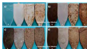
Figure 2. Effect of composting on the aspect of (a) neat PLA and the composites: (b) PLA–agave, (c) PLA–coir, and (d) PLA–pine.
