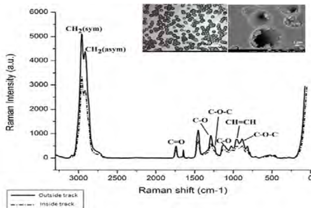
Figure 1. Raman spectrum inside and outside of the track.
