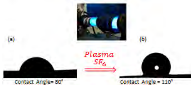
Figure 1. Drop of water on a paper sample: a) wetting surface and b) non-wetting surface (hydrophobic).
