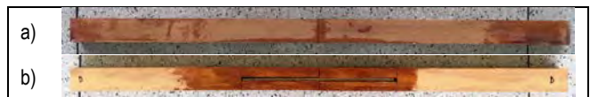
Figure 1. Wood specimens: a) Sample with a joint glued at the center, b) Sample with a joint at the center and reinforced by sisal/epoxy composite
